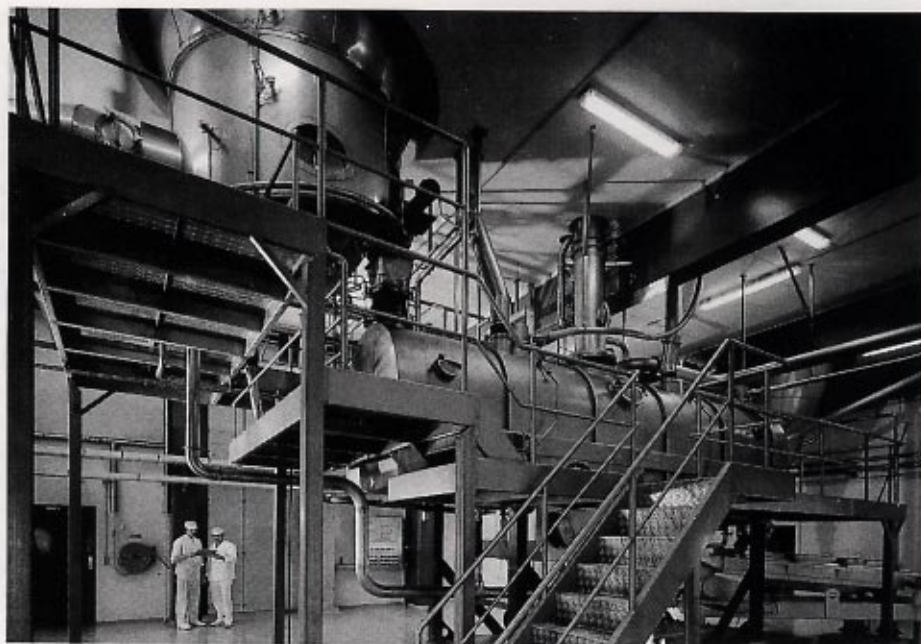
Vibrating fluid bed for agglomeration of food powders.
