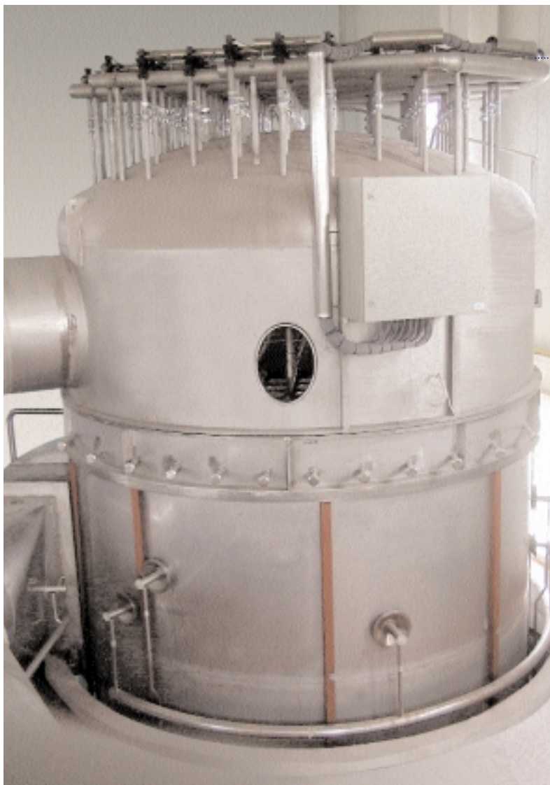
Niro's SANICIP™ CIP-able Bag Filter installed at Mokate's new plant in Poland.
