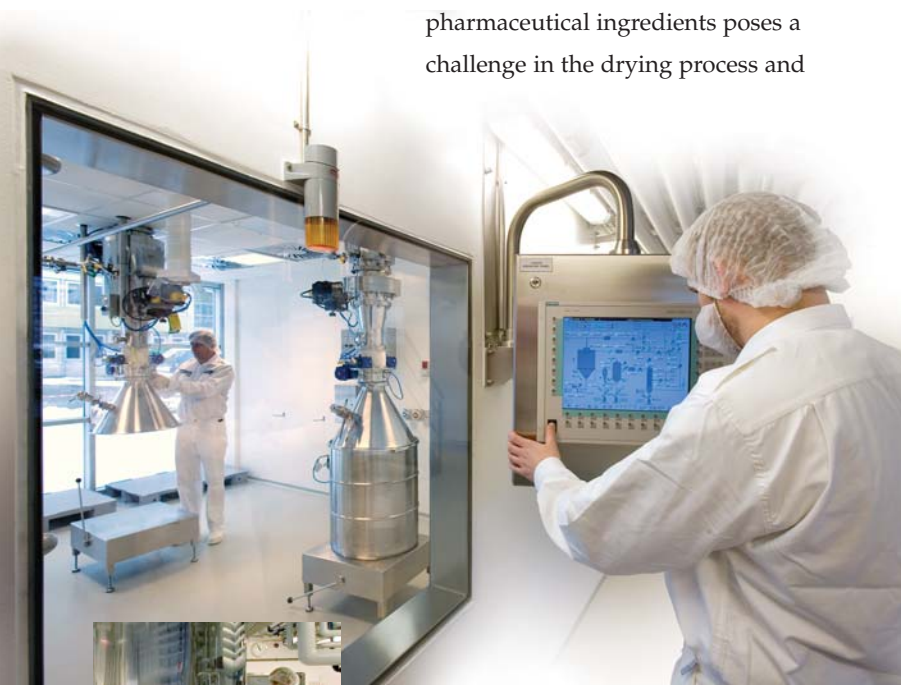
GMP facility including a PSD-4 spray dryer operating in closed cycle mode
