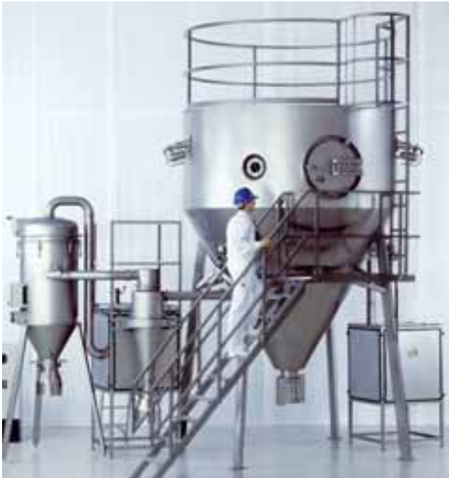
VSD-6.3-R, designed for rotary atomization. Drying chamber size: Ø 2500x1000 mm, 60° cone.
