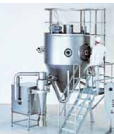
VSD-6.3-P with rotary atomizer, cyclone and exhaust fan in noise attenuation box. Drying chamber size: Ø 1600x800 mm, 60° cone.
