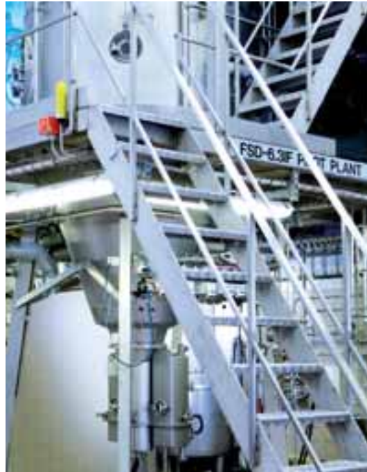
FSD™-6.3 with triple chamber static fluid bed. Installed in Niro Test Center, Copenhagen. Drying chamber size: Ø 1600x800 mm, 40° cone.
