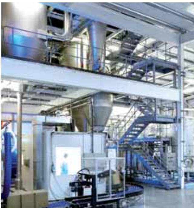
VSD-50-N, designed for co-current pressure nozzle atomization. Drying chamber size: Ø 3200x4500 mm, 60° cone.
