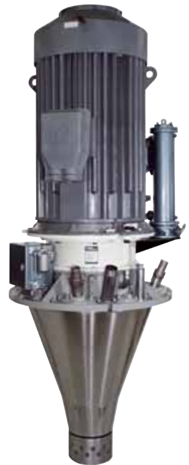
A single rotary atomizer can treat the flue gas from a 450 MW e unit.
