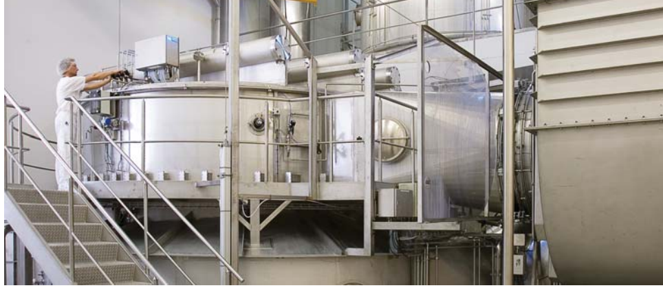
The top of a SANICIP™ bag filter
