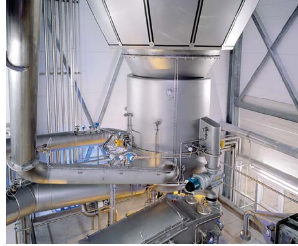
Chamber cone, integrated fluid bed and sieve with CIP nozzles
