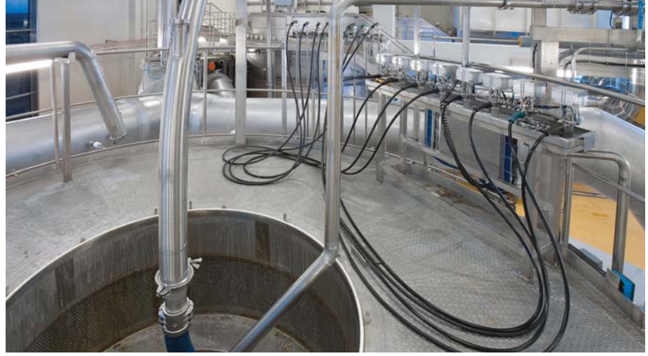
Spray drying chamber in CIP mode. Atomizer nozzles removed from atomization zone. A CIP turbine cleans surface of inner chamber walls
