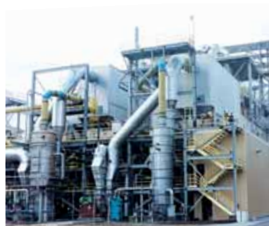
Niro CONTACT FLUIDIZER™ with integrated filters for the production of dense soda ash
