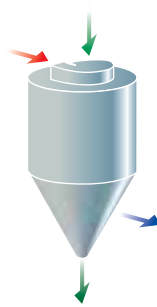
3. Co-current, conical base with rotary atomizer, for both heat-sensitive and stable products.
