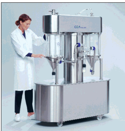
The latest of Niro's mini-processors – the SDMicro™ spray dryer for extremely small capacities within chemistry and pharmacy.
