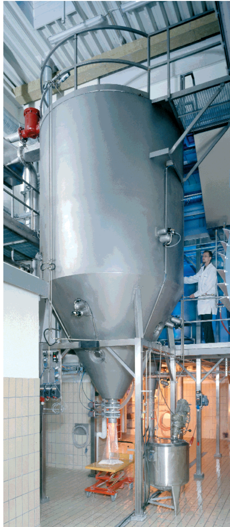
The latest of Niro's mini-processors – the SDMicro™ spray dryer for extremely small capacities within chemistry and pharmacy.
