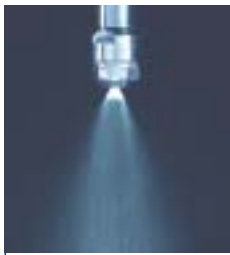
Pressure nozzle atomizer in operation
